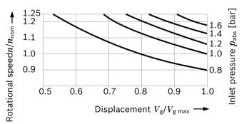
The inlet pressure is the static supply pressure and the minimum dynamic value, respectively, e.g. in case of pre-charge pressure.
